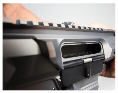
RELEASE THE CHARGING HANDLE ALLOWING THE BOLT CARRIER ASSEMBLY TO TRAVEL FORWARD UNDER SPRING TENSION FROM THE BUFFER SPRING.
