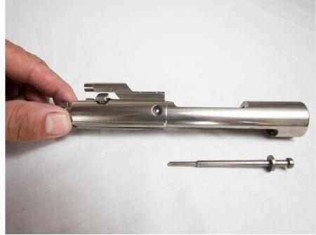
INSTALL THE FIRING PIN INTO THE BOLT AND PUSH FULLY FORWARD. USE THE FIRING PIN RETAINING PIN TO SECURE THE FIRING PIN IN THE BOLT CARRIER ASSEMBLY.
