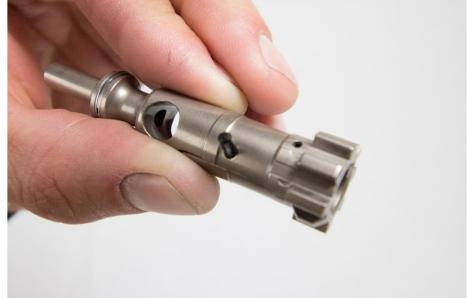
INSERT THE BOLT INTO THE BOLT CARRIER ASSEMBLY. BE SURE TO ALIGN THE BOLT PROPERLY WITH THE EXTRACTOR FACING THE RIGHT SIDE OF THE BOLT CARRIER.
