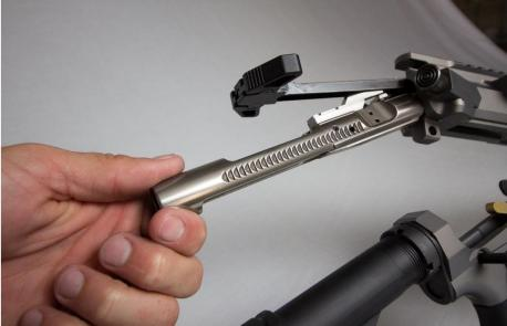
REMOVE THE CHARGING HANDLE BY ALIGNING THE EARS ON THE CHARGING HANDLE WITH THE CORRESPONDING CUTOUT IN THE UPPER RECEIVER.
