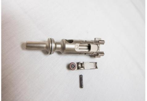
THE RIFLE IS NOW FIELD STRIPPED AND READY FOR CLEANING. USE A QUALITY SOLVENT TO REMOVE ANY PRESERVATIVE FROM ALL METAL SURFACES. BE SURE TO CLEAN THE BORE USING SOLVENT SOAKED PATCHES. FOLLOW THIS CLEANING WITH AN APPLICATION OF A QUALITY OIL OR LUBRICANT DESIGNED FOR FIREARMS USE.
