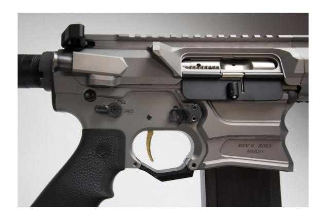
WHILE HOLDING THE WEAPON IN A SHOOTING GRIP, ROTATE THE SELECTOR LEVER TO THE "SAFE" POSITION. WITH THE SELECTOR ON SAFE, PULL THE TRIGGER TO THE REAR. THERE SHOULD BE NO MOVEMENT OF THE TRIGGER AND THE HAMMER SHOULD NOT BE RELEASED.
